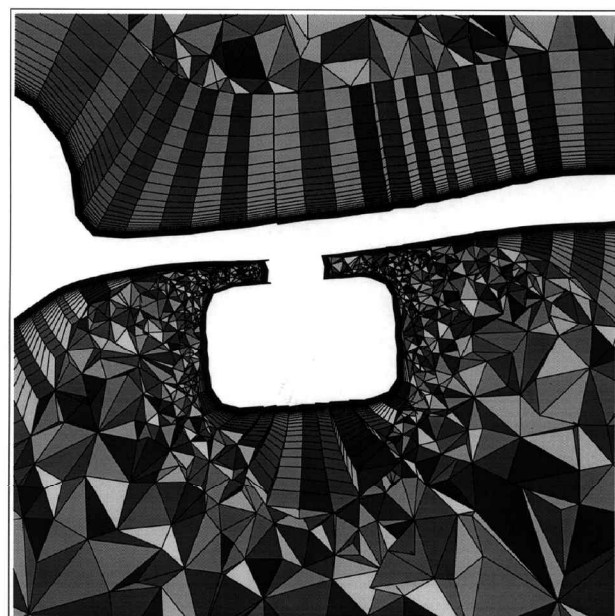
Fig. 18 Closeup of the hybrid grid for the HSCT aircraft around the engine cavity. The tetrahedral mesh is very dense here compared to other regions so as to match the thin local prism cell sizes.
