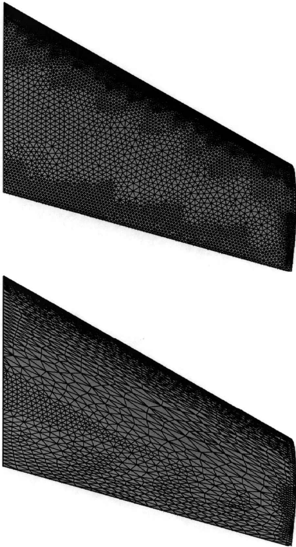
Fig. 12 Significant savings in number of triangles are realized because of the use of leading and trailing edge line segments for the M6 wing. The top mesh is an isotropic mesh with 39,290 faces. The bottom mesh is an anisotropic mesh with 6333 faces. Note that even though the isotropic mesh has six times the number of faces, the anisotropic mesh has the same chordwise point distribution.
